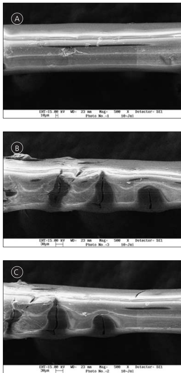
FIGURE 2. SURFACE STRUCTURE OF POLY(DIMETHYL SILOXANE) (PDMS) FIBER, AS OBTAINED BY SCANNING ELECTRON MICROSCOPY (500-FOLD MAGNIFICATION). (A) BEFORE ASSAY; (B,C) AFTER 3 RD REMOVAL WITHOUT RETRACTING THE FIBER.
